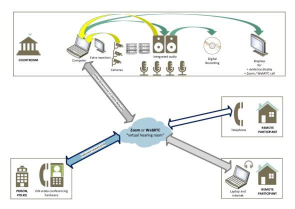
Integrated audio system with cameras, displays and visual processing. Requires one computer to join the video meeting – but connects all of the cameras, displays and audio system to that computer, allowing everyone in the courtroom and in the remote meeting to see and be seen, and to hear and be heard.
