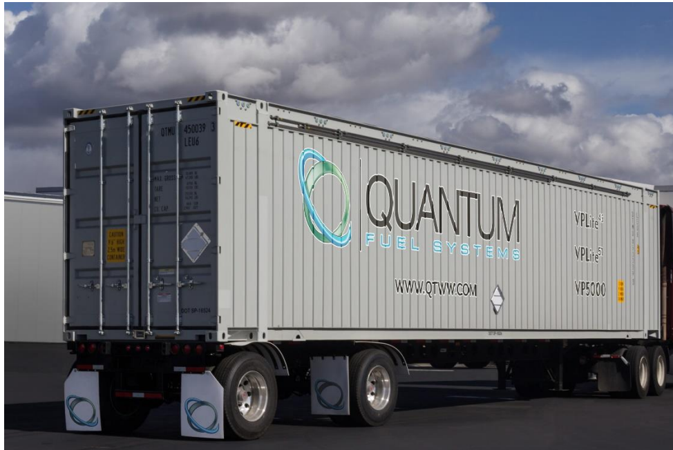
Figure 5: Tube Trailer to Transport Hydrogen Fuel (Markham to and from Mississauga)
