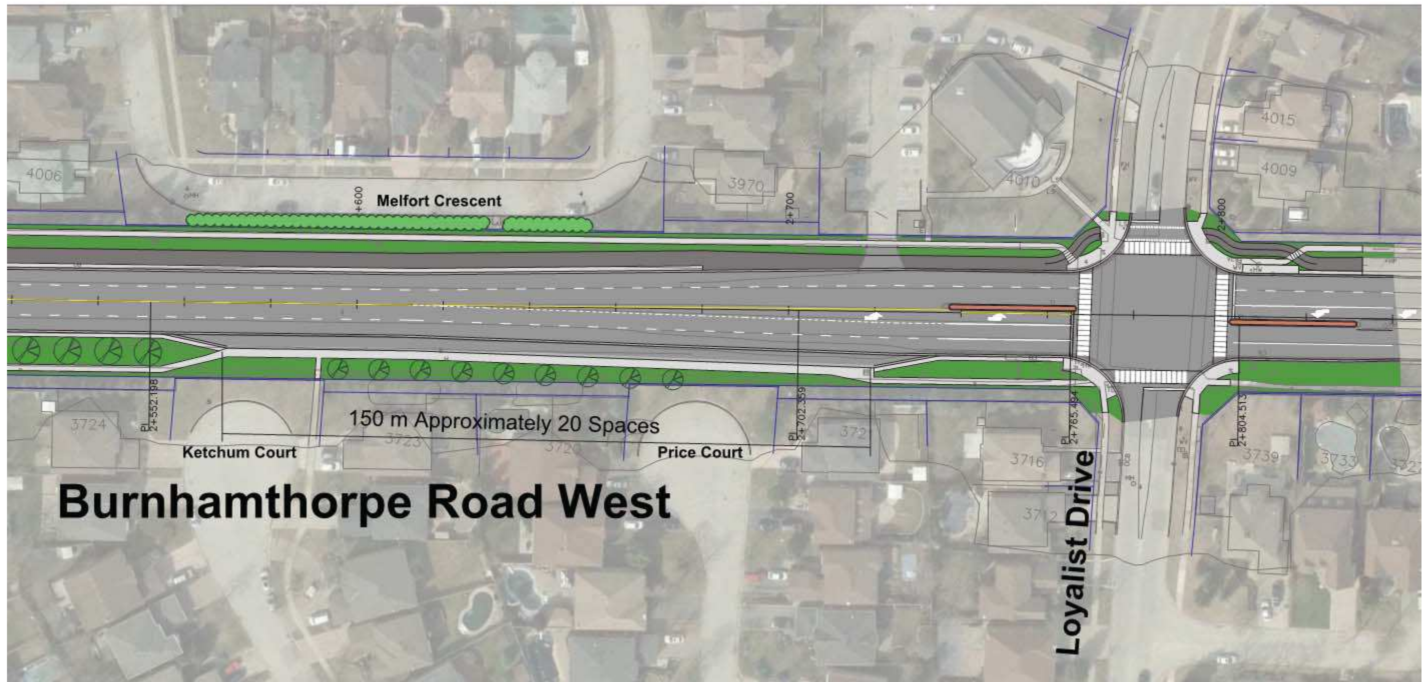
Figure 3: Alternative Design Concept #3 - Widen Burnhamthorpe Road West to 4 Lanes with In-Boulevard Parking on the South Side
