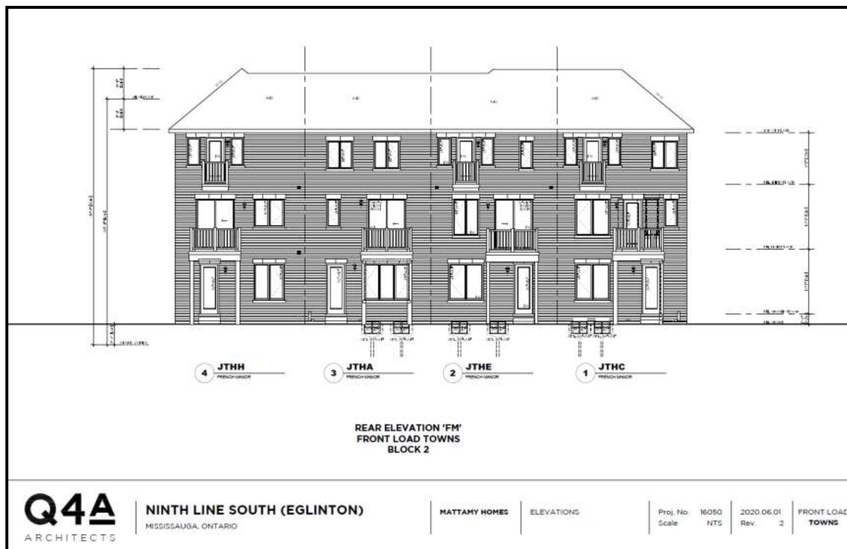
Figure 17: Front Load Towns (French Manor), Block 2 – Rear Elevation (Q4A Architects 2020a)
