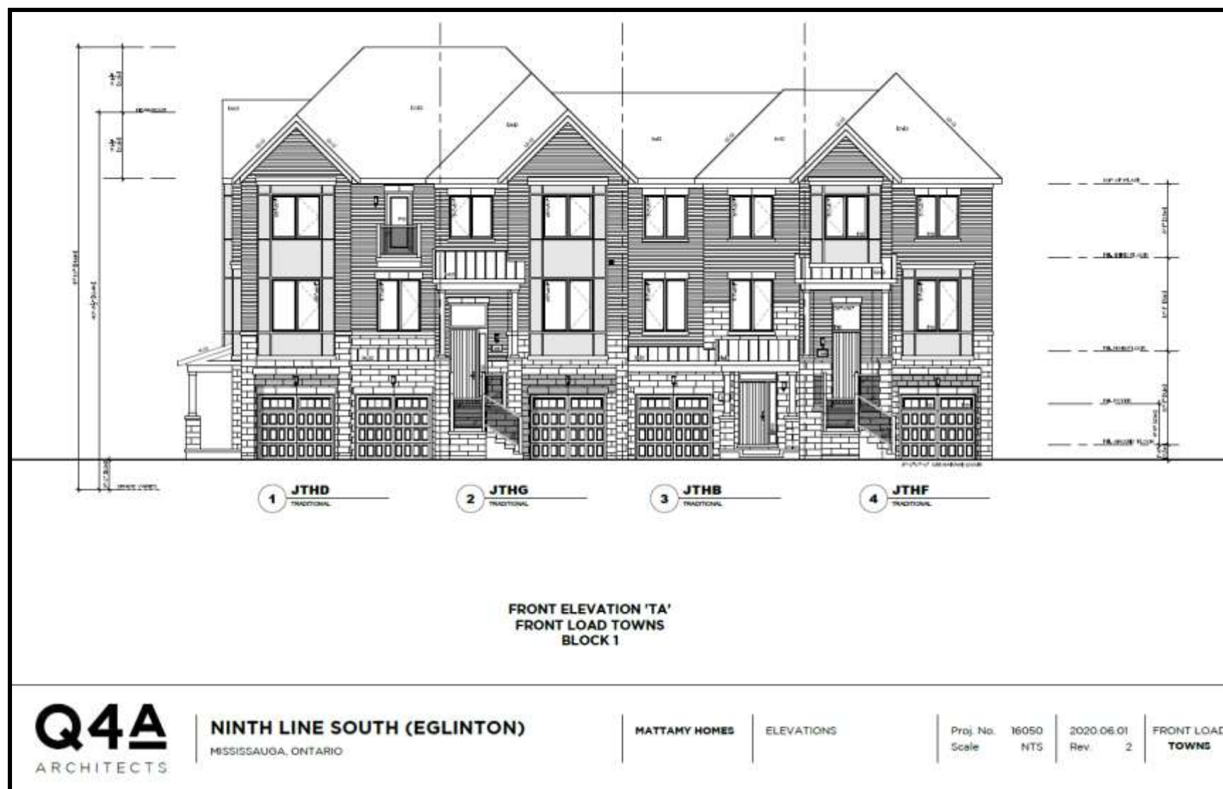
Figure 19: Front Load Towns (Traditional), Block 1 – Front Elevation (Q4A Architects 2020a)
