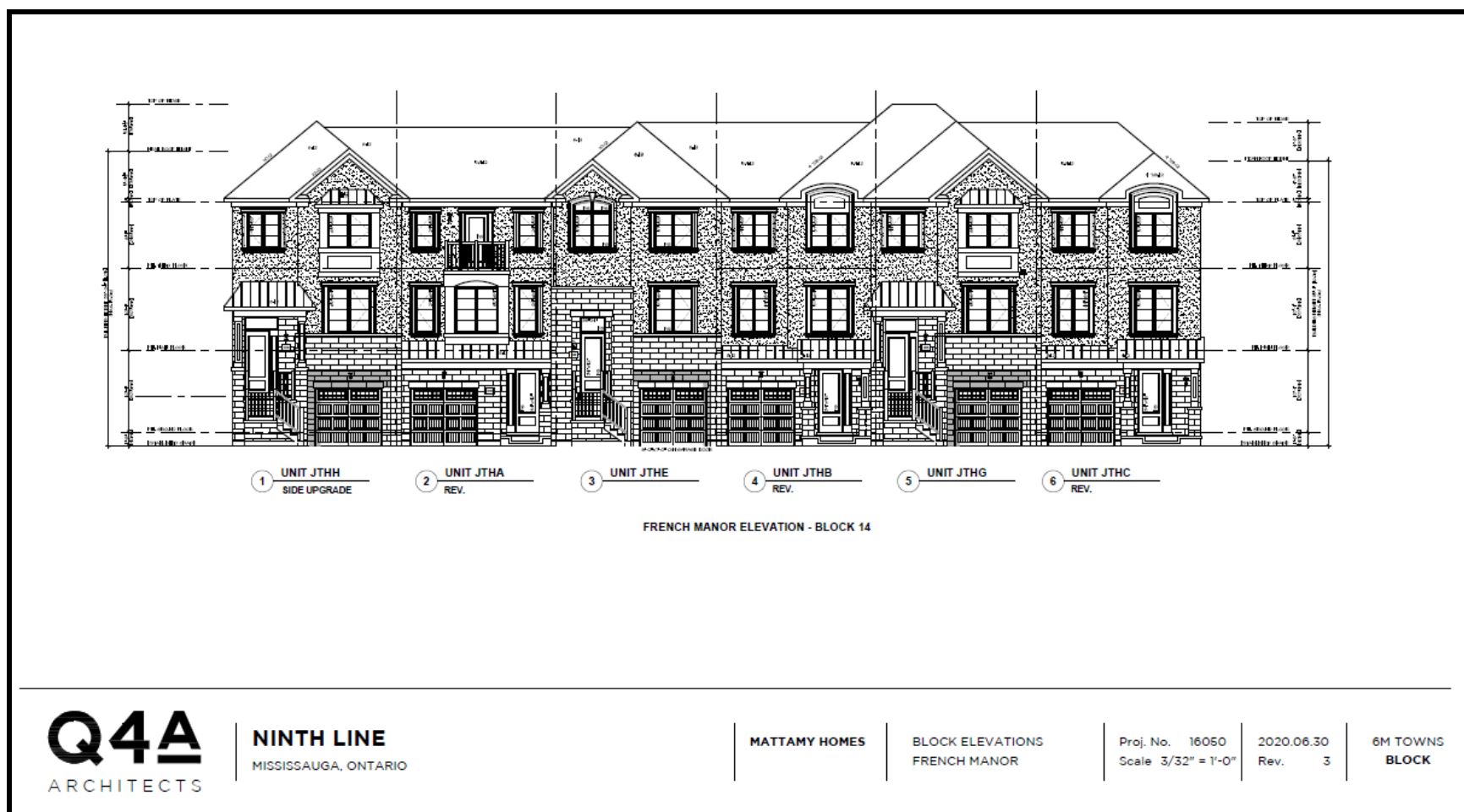
Figure 33: Village Homes (French Manor), Block 14 – Front Elevation (Q4A Architects 2020b)
