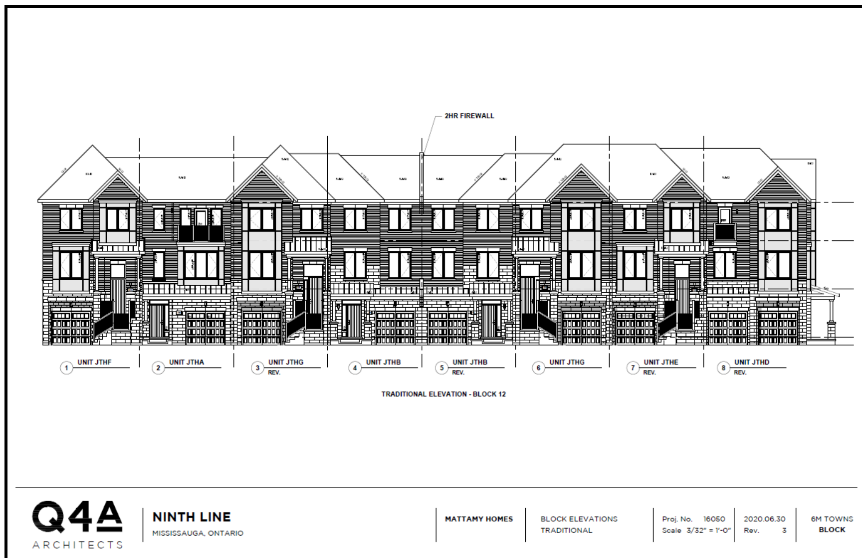
Figure 25: Front Load Towns (Traditional), Block 12 – Front Elevations (Q4A Architects 2020b)
