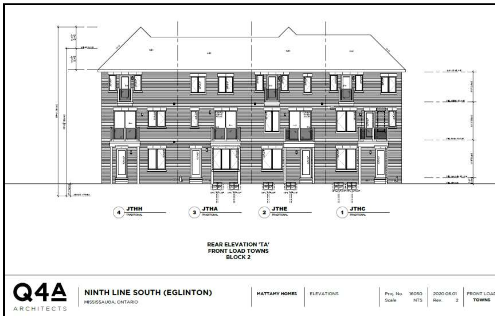
Figure 23: Front Load Towns (Traditional), Block 2 – Rear Elevation (Q4A Architects 2020a)
