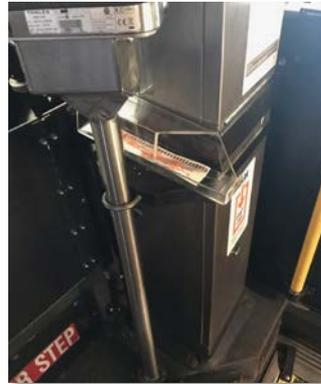
Paper transfer chutes designed and installed in-house
