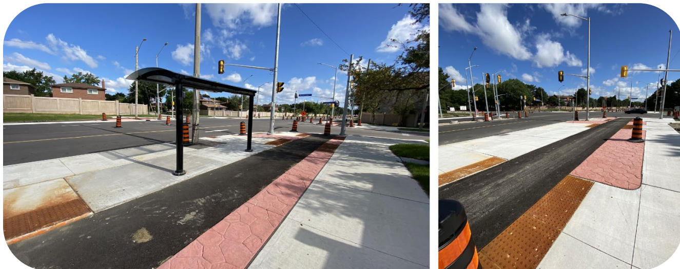
Figure 3: Mixing Zone - Preferred configuration example at Rathburn Rd. and Rockwood Rd.
