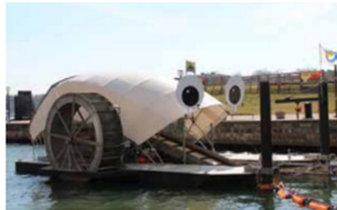
The Inner Harbor Water Wheel in Baltimore Harbor (Trash Collecting Wheel)
