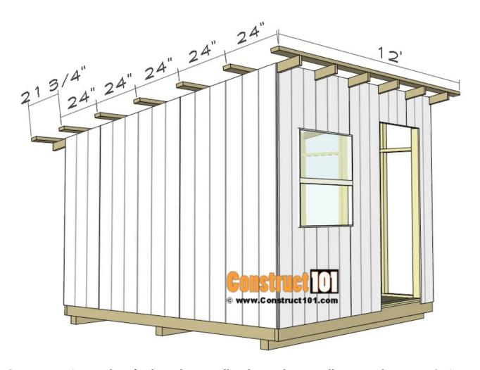
Cut seven  $2\times4$ 's to 12' long for the purlins. Install purlins as shown on illustration above using  $3\ 1/2''$  nails.
