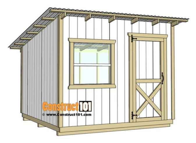
Measure and cut  $1\times4$ 's to size for the corner and window trim. Install the  $1\times4$  trim using 2'' finishing nails.
