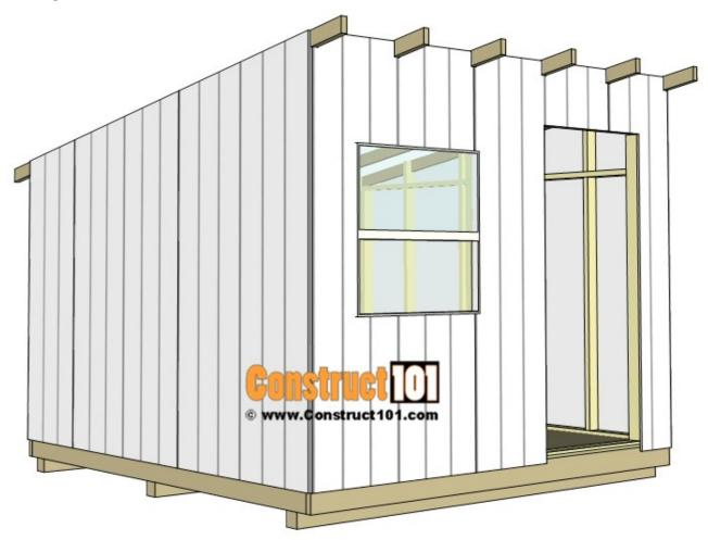
Measure and cut the t1-11 exterior siding to size, notch front and back siding around rafters. Install siding using 2" finishing nails.
