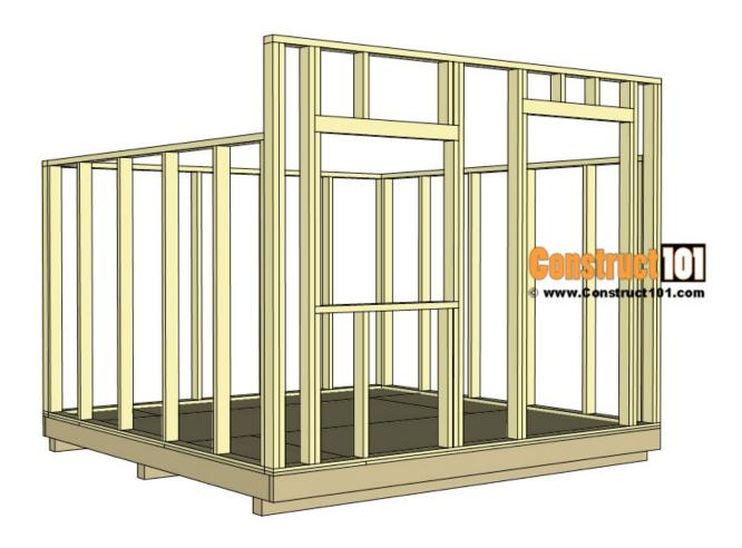
Secure the wall frames using 3  $1/2^{\prime\prime}$  nails.
