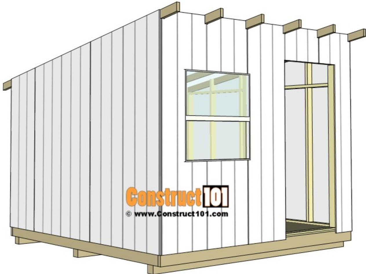
Measure and cut the t1-11 exterior siding to size, notch front and back siding around rafters. Install siding using 2" finishing nails.
