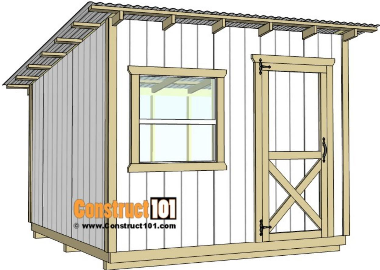
Measure and cut 1×4's to size for the corner and window trim. Install the 1×4 trim using 2" finishing nails.
