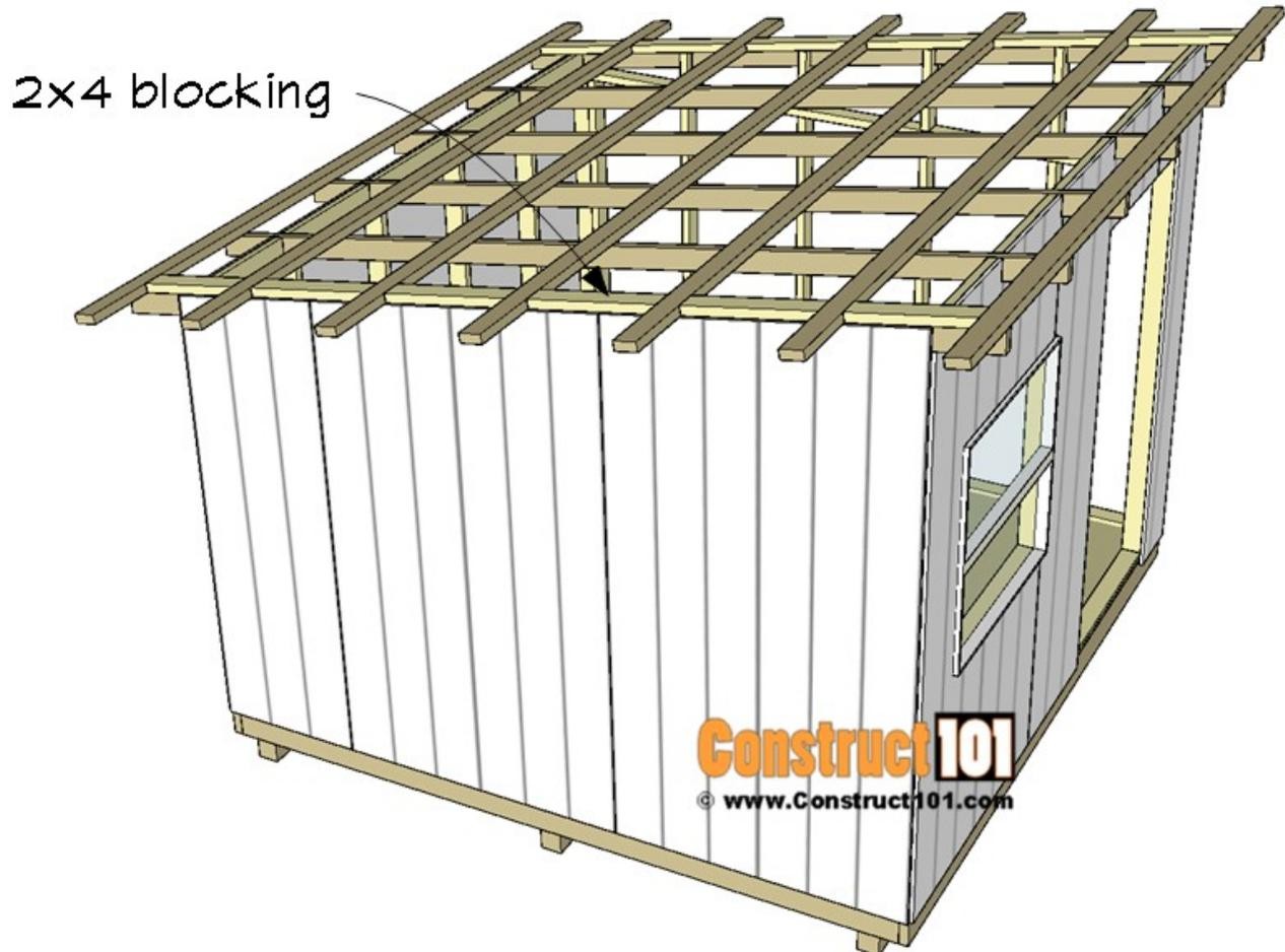
Measure and cut 2×4 blocking and install between the purlins using 3 1/2" nails
