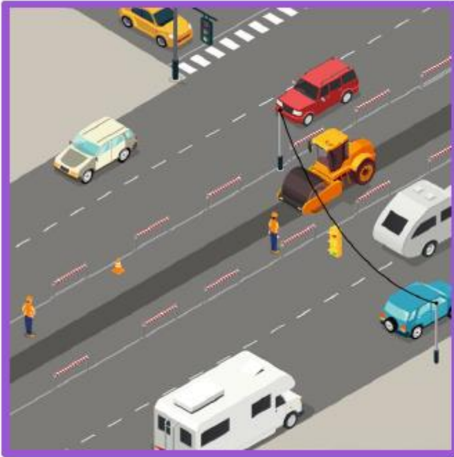
Stage 1: Median removals and installation of temporary traffic signals.
