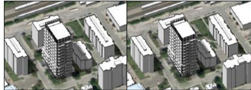
Renderings of the subject proposal and the sun/shadow impacts in June (left image) and December (right image)
