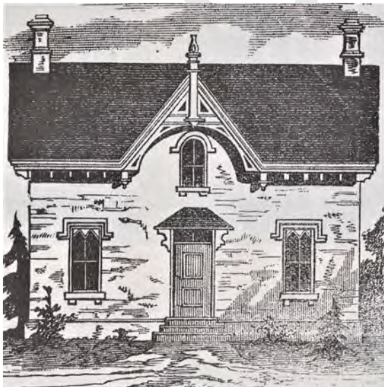
GOTHIC REVIVAL STYLE COTTAGE – a popular style for rural residences in Ontario from the 1850s-70s [ The Canadian Farmer , 1865] – 3 bays by 2 bays wide, with the front entrance on the long elevation below the gable and chimneys on the end walls
