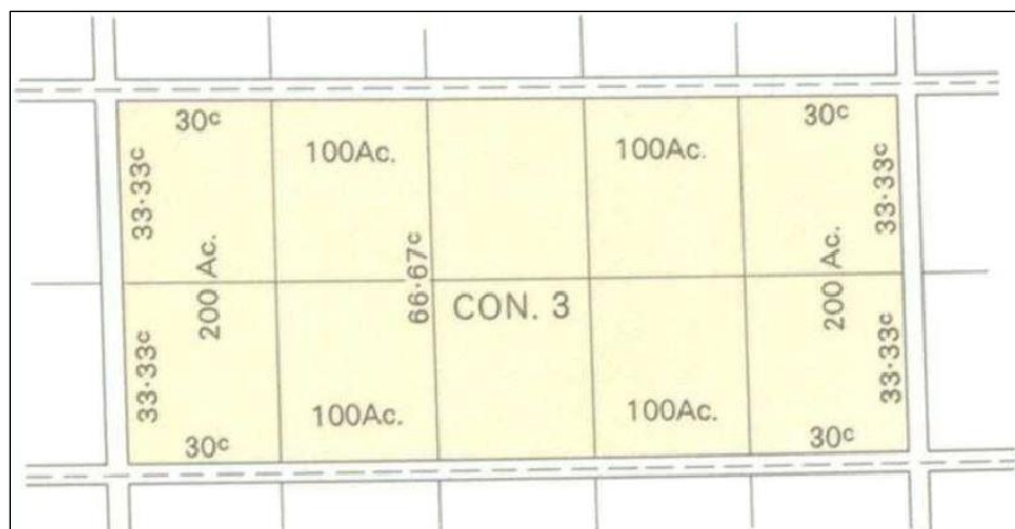
Plate 3: Double-front survey system (Dean 1969)
