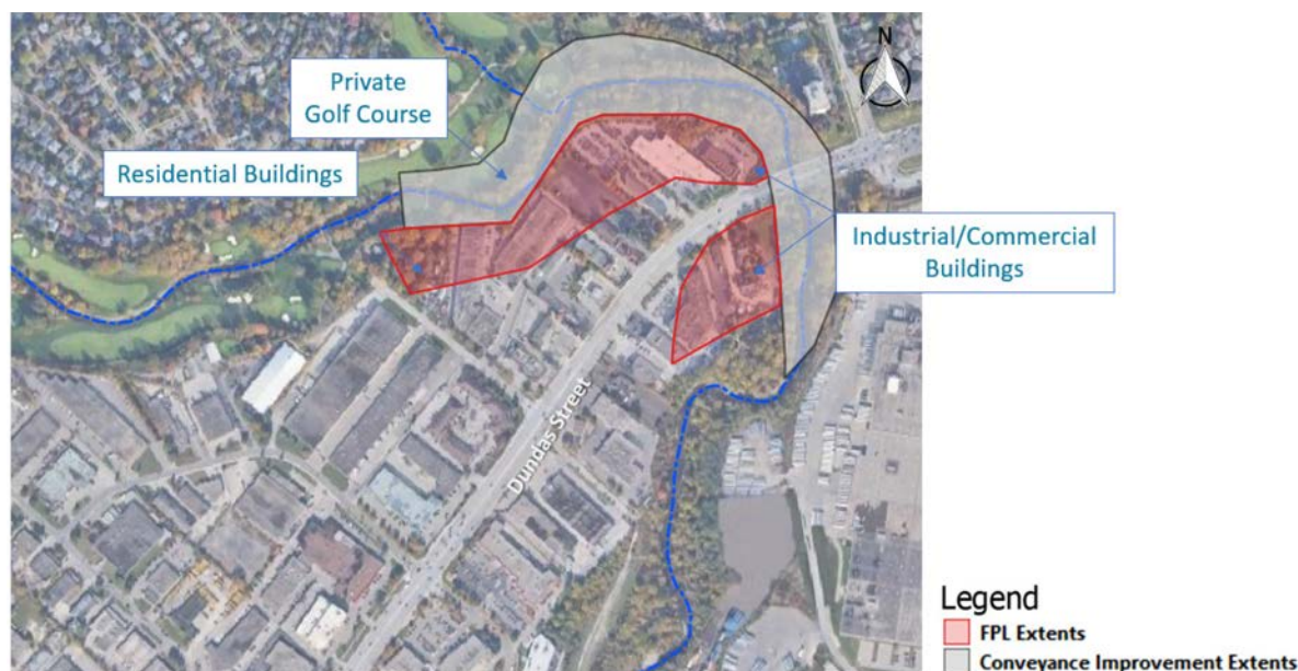
FIGURE 11 Flood Protection Landform and Floodplain Improvement Extents and Property Acquisition
