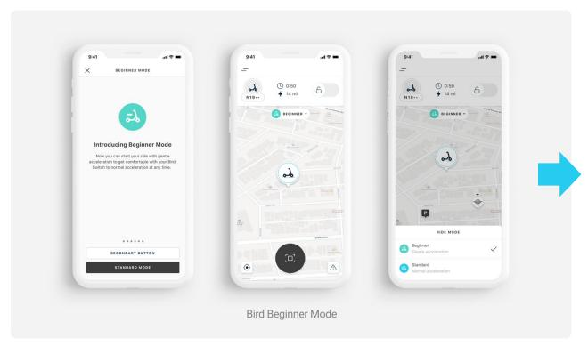
A feature that automatically **softens** an e-scooter's acceleration, allowing riders to **slowly work their way up** to full speed.
