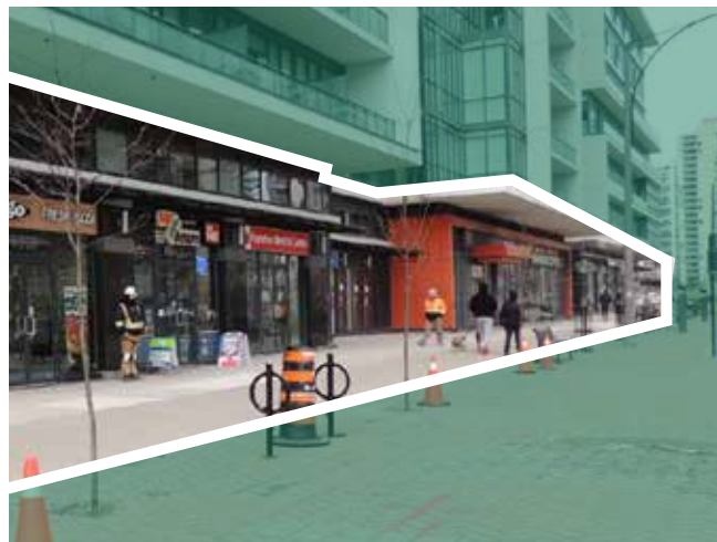
Figure 12: Ground floor conditions on all A - Streets. Balconies should be inset and any canopy projections should be between 2 and 4 meters.
