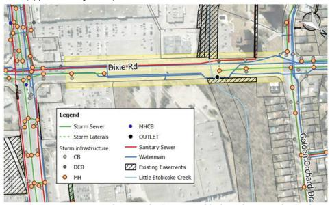
Figure 1 – SUE Investigation and Topographic Survey up to 20m beyond Dixie Road right-of-way limits. Approximate limit outlined in yellow.
