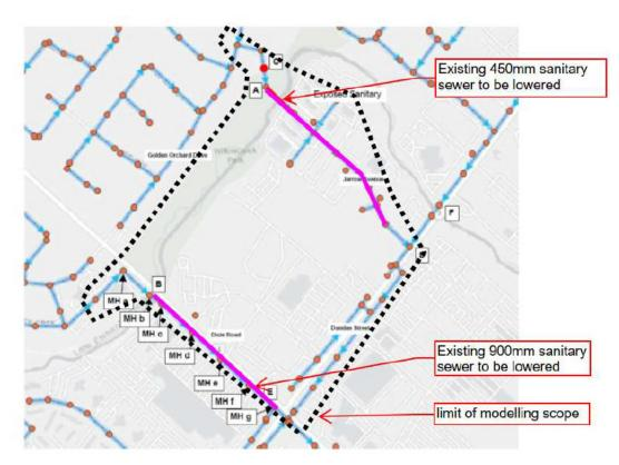
FIGURE 1 Sanitary Sewer Relocations Overview
