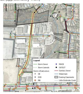
Figure 2 – SUE Investigation and Topographic Survey up to 20m beyond Jarrow Avenue right-ofway limits. Approximate limit outlined in yellow.
