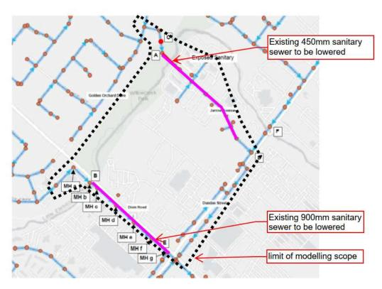
FIGURE 1 Sanitary Sewer Relocations Overview
