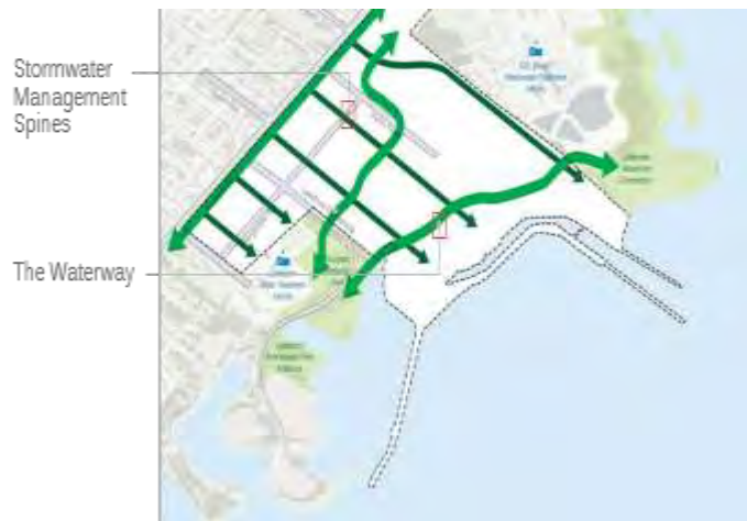
Figure 6: An innovative approach to stormwater management - series of north-south and east-west spines adds natural elements to the public and private realm while providing an important water collection function.
