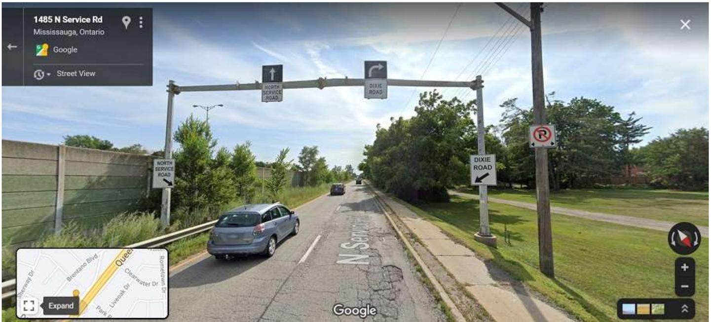
**Photograph 6:** The right lane gets a warning for the northbound slip lane to Dixie Road. No warning at all for the left lane NSR exit which is far more dangerous.
