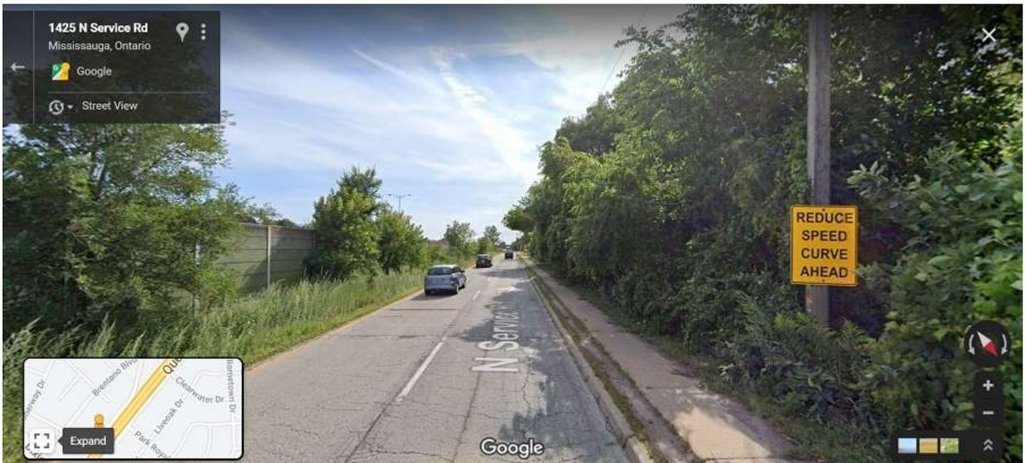
**Photograph 8:** The right lane gets a second, strong warning for the northbound slip lane to Dixie Road. No slow-down warning for the imminent left lane exit at NSR.
