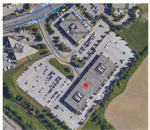
The blue lines are our fiber cable/duct, the orange is our copper cable, the green is a manhole, and the yellow is a copper pedestal.
