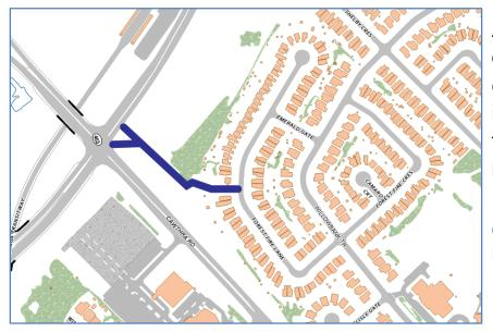
A new multi-use trail on the east boulevard of Cawthra Road is under construction. It connects the Eastgate Parkway intersection and Cawthra Transitway station to an existing walkway into the neighborhood.
