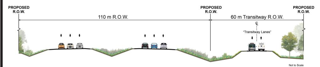
The corridor will initially be designed as a 6-lane highway with a posted speed limit of 110 km/hr, with the potential for expansion to 10 lanes.
