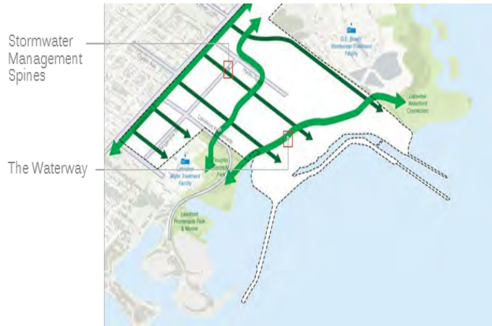
Figure 13.5. An innovative approach to stormwater management - series of north-south and east-west spines adds natural elements to the public and private realm while providing an important water collection function.
