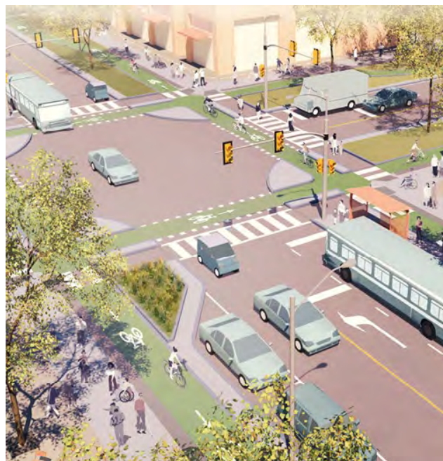
Figure 7.2. Multi-modal transportation is a primary feature of complete streets , as shown in this demonstration.
