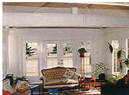
The interior of the sunroom addition. The owner has used elements to complement what is seen in the original building, such as the beams/rafters along the ceiling (similar to what is seen in the dining room and study photos) or the windows being divided with muntins rather than being one solid piece of glass.
