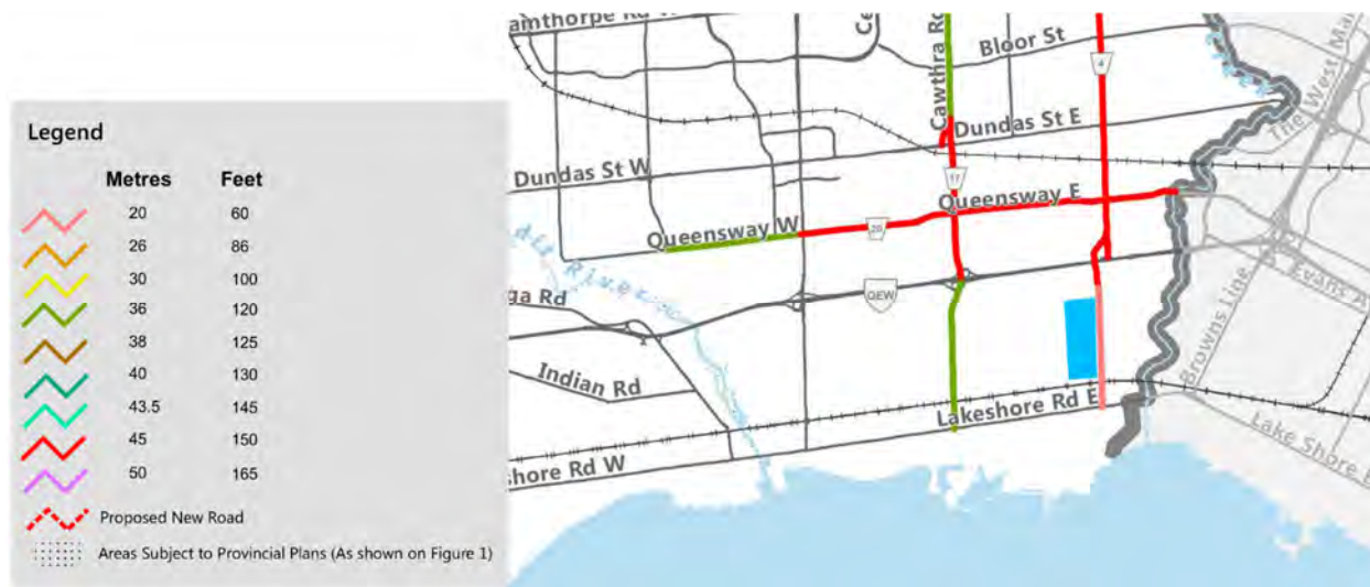
Image 2.3.13: Annotated excerpt from Region of Peel Official Plan, Schedule F-3, showing a 20-meter Right-of-Way along Dixie Road adjacent to the Lakeview Golf Course.
