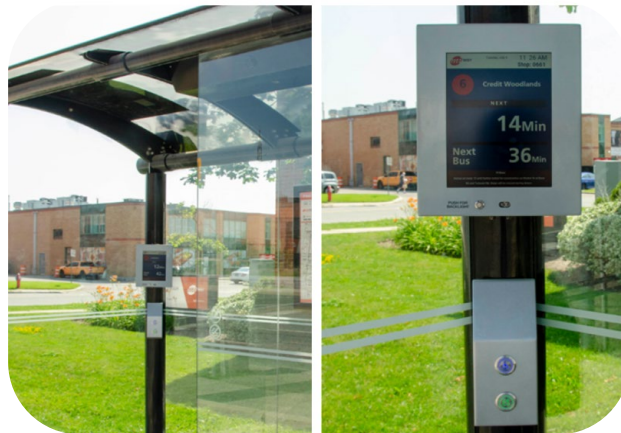
Figure 10: 10-inch reflective, solar powered, LCD model, displays in colour and option to display a high-contrast version with larger text.
