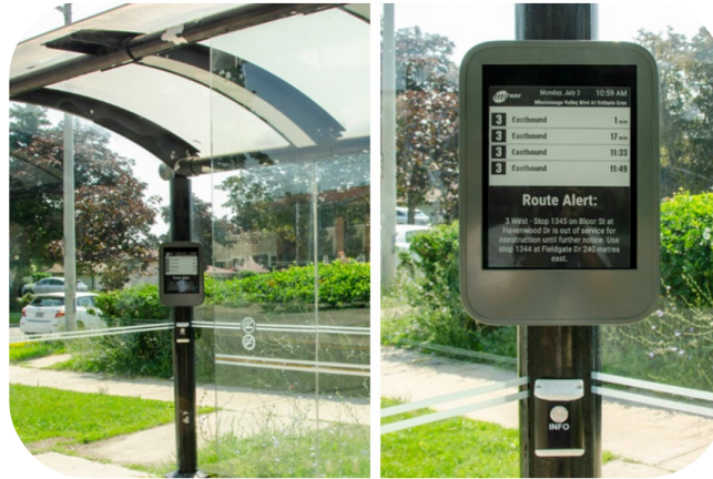
Figure 9: 13-inch E-Ink model that displays information in black and white with high contrast.
