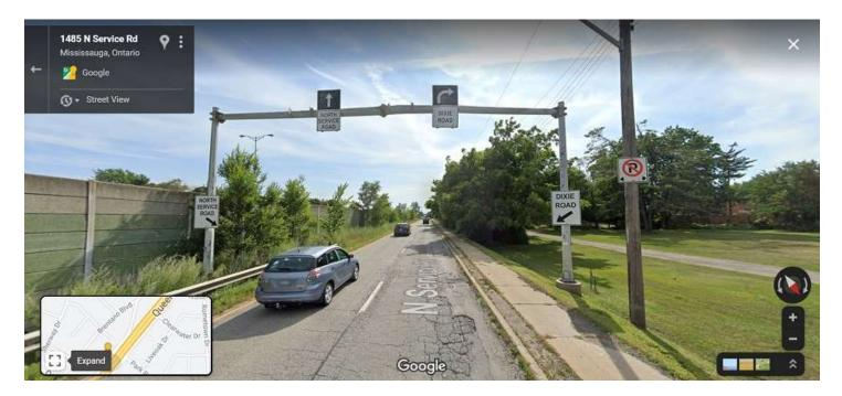
**Photograph 6:** The right lane gets a warning for the northbound slip lane to Dixie Road. No warning at all for the left lane NSR exit which is far more dangerous.
