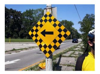
**Photograph 18:** Heavy vehicles come off the QEW Dixie off-ramp at high speed. The small stop sign set so far back, and the ambiguous warning signs and flashing light further on and up the pole, beyond a cyclist's view while attempting to navigate the turn, don't convey the extreme danger that could arrive at any minute. Ironically, the eastbound traffic side has all the signs and warnings but misses the point.
