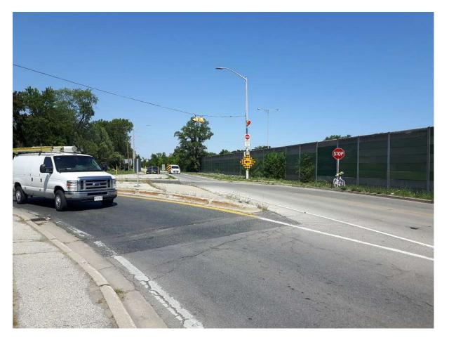
**Photograph 17:** From the set-back position at the stop sign on eastbound NSR, with obstructing eye-level signage at the corner, it is hard to even see the oncoming traffic.
