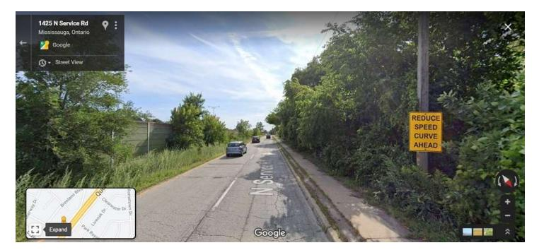
**Photograph 8:** The right lane gets a second, strong warning for the northbound slip lane to Dixie Road. No slow-down warning for the imminent left lane exit at NSR.
