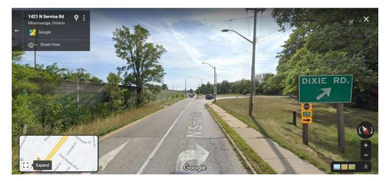
**Photograph 10:** Lots of way-finding signage for the right lane. Nothing at all for the left lane NSR exit which looks benign, with no stop nor warning of local traffic that may cross the path unexpectedly. The onus is placed on local traffic to stop and yield to the oncoming higher-speed traffic, rather than the other way around. A turning NSR driver or cyclist could misjudge time needed to clear the innocuous-looking QEW exit lane.
