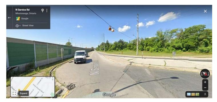
**Photograph 16:** A wider view shows how far the stop sign is from the danger lying ahead. A cyclist might think that once past the stop sign, it is clear sailing. "Do not Enter" symbol seems small and routine, "Keep Turning" (checkered diamond) seems clear, but the "Opposing Traffic has Right of Way" statement, which must be read, up so high, is inadequate to convey the severe danger of oncoming high-speed traffic.
