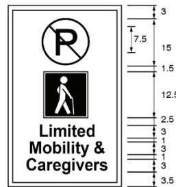
Figure 94: Type-C Parking Signage
