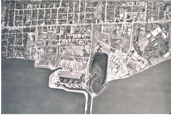
Fig. 14 Ralph Crysler, "Lakeview Generating Station, Aerial Photo," 1972, City of Mississauga Historic Images Gallery, Lakeview Gallery, LG_R196.jpg. The photograph is centred on the station's intake channel, powerhouse and coal yard. North of the station, along Rangeview Road and Lakeshore Road East, are factories. Immediately to the east is the sewage treatment plant. Farther east are the former buildings of Small Arms Limited.
